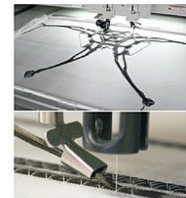
Preform production with 1700 mm x 1500 mm by TFP-Technology
