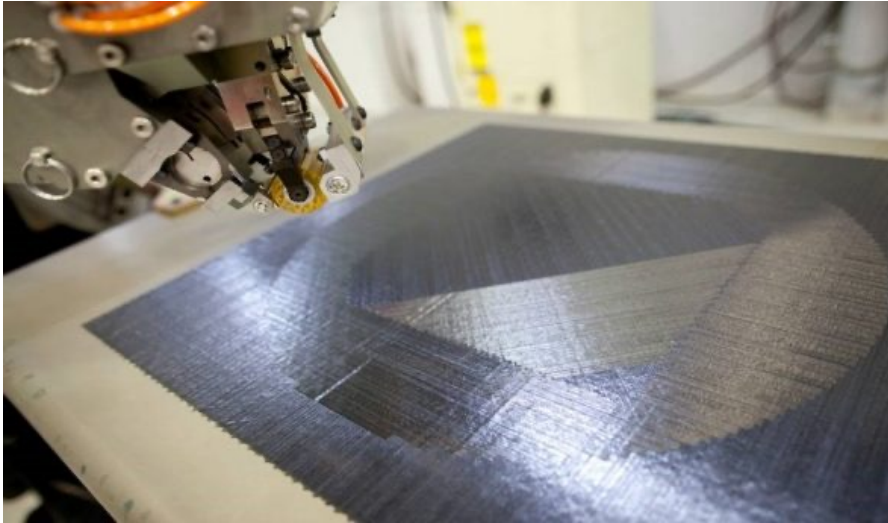
Multiple layers with predefined angles (thermoset AFP)
