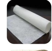
Consolidation by thermobonding of a non-woven structure obtained by carding/needling and containing thermofusible fibres.
