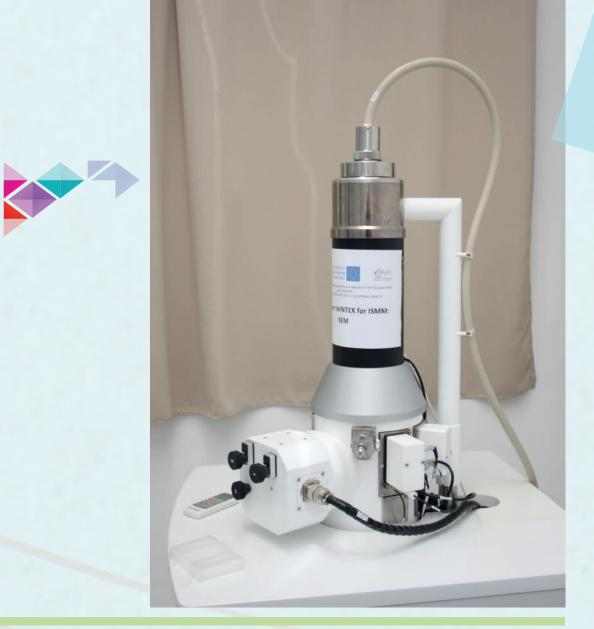
Since its appearance, the scanning electron microscope (SEM) has proven to be a powerful tool for characterizing materials, in particular for the surface shap, topography, grain size of metals, observation of defects (cracks, damage, fractures, etc...) porosity, shapes and distribution of charges in polymers, observation of nanomaterials or biological cells.
